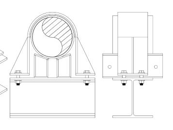
**CUSTOM BUILT PIPE SUPPORTS TO MEET SPECIFICATIONS**
